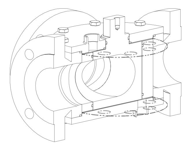
Another option that can be used for slurry applications consists of a valve that utilizes a rotor with round seals. This allows us to place a sealing o'ring between the rotor and the caps minimizing the internal volume that particles from the slurry can get into. The caps are modified to accommodate the o'ring and thrust washers that keep the rotor centered. Also, the seals have an additional diameter o'ring to prevent particles from the slurry from getting in behind the seals.
